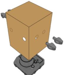
Place your Jellyfish on the vibrating body and fix it using Recyclips.
