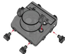
1 Install the Recyclips™ on the vibrating unit as shown in the figure.
